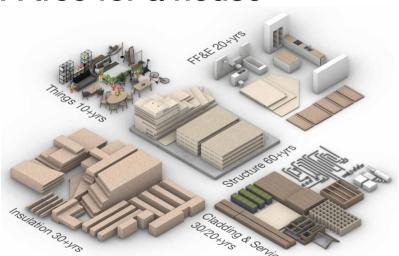
Diagram 3: A kit-of-parts approach to manufacturing A typical family home is laid bear. Made from a single mature spruce, each element holds a different service life; therefore designing for disassembly allows for circularity.
